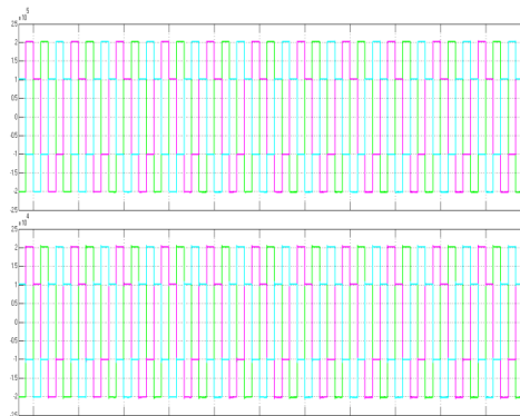
Figure: 4.11 voltage and current output waveform for SPWM inverter
